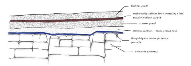
Figure 2.3: Limestone pavement protection system
