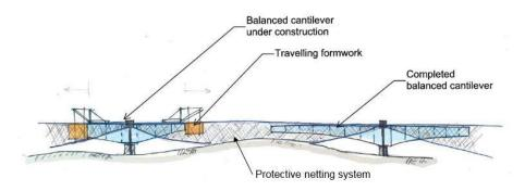
This is a less invasive construction methodology as it avoids any large scale construction works off the Limestone pavement, although, some parts of the bridge will be constructed using Construction Method 1. A netting system will also be used over the Limestone pavement and Turlough area to catch any falling debris or materials. This will ensure that no damage occurs to the Limestone pavement environment beneath.
