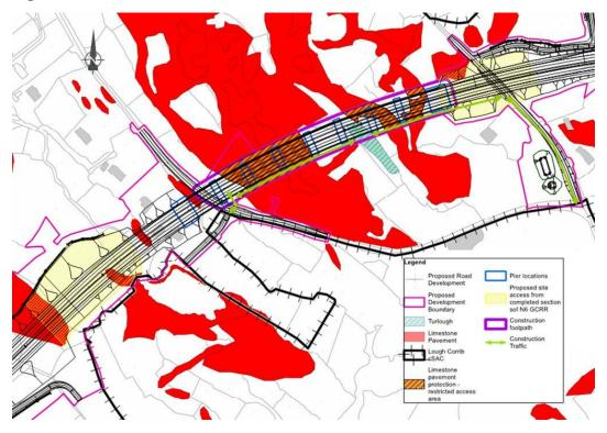
Figure 3.1: Construction Method 2 Site Access
